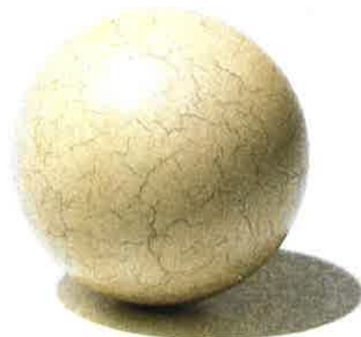
This 19th-century billiard ball was made from celluloid, an early plastic that replaced elephant ivory—which was already growing scarce.
