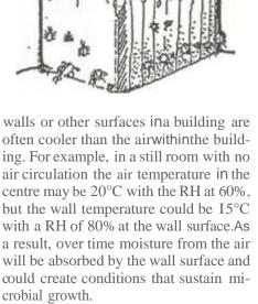
To determine if microbial growth is possible or not, it is necessary to know at what relative humidity the air is in equilibrium with **a** given moisture content in a material. For any material, this equilibrium relative humidity is referred to by scientists as its 'water activity' (a..). Air and surface temperatures have a bearing on the moisture content and the a .
