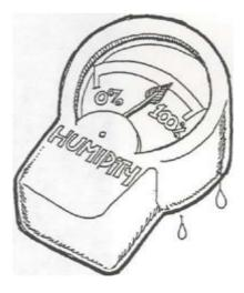
Resistive hygrometers havesensors that use eithersalt-saturated filaments or metal grids embedded in a casing. The resistance of the probe varies with the amount of moisl'lm .The vol Lage or current passing through the probe is a function of the
