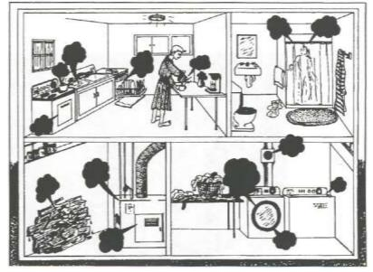
Figure 2.-Common indoor moisture sources.
