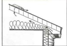
Figure 5.-Passive attic vents.
