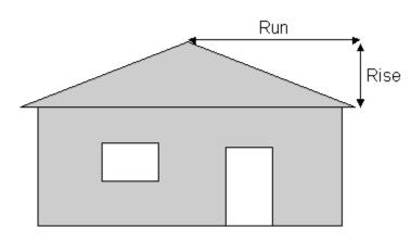
Roof pitch is measured in terms of vertical rise over horizontal run. In other words, a 2 in 12 pitch means that for every 12 feet of width to the home, the peak of the roof is 2 feet higher than the eave. Keep in mind that roof pitch indicates a peaked or pointed or gabled roof, not a rounded roof.
